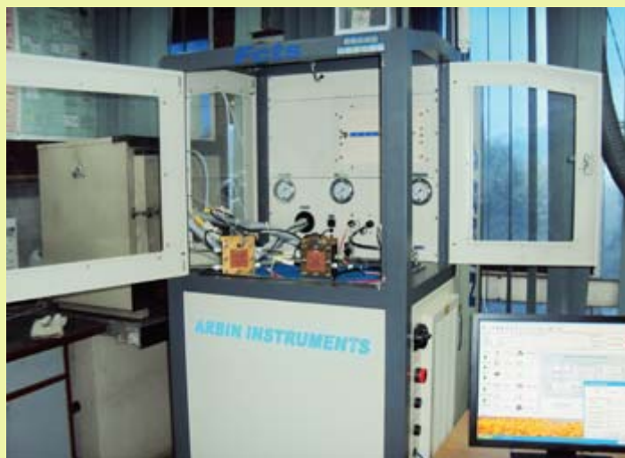
Fuel Cell test station set up at IIT Delhi under a R&D Project sponsored by the Ministry
