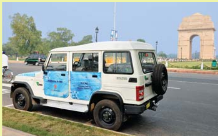
H-CNG vehicle undergoing field trials
