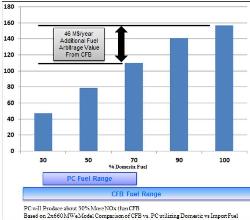
**Figure 5. Plant Operating Cost Savings as Domestic Fuel Utilization Increases (M\$/Yr)**
