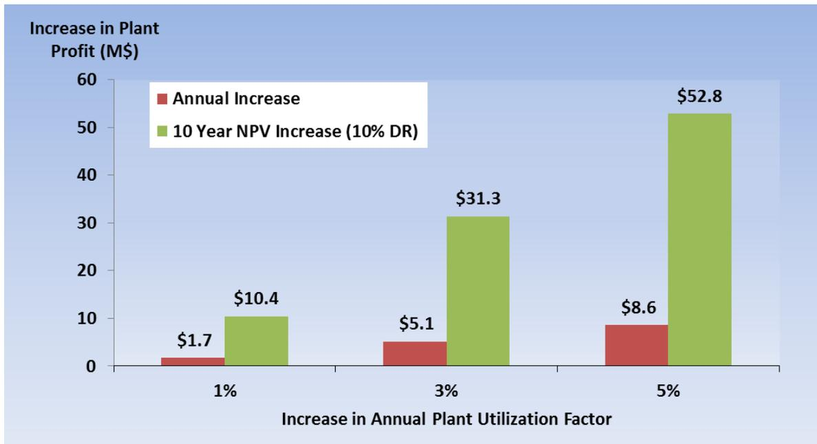
**Figure 6. Results from power plant proforma analysis based on 60\$/MWe electricity tariff, 30 \$/tonne coal, and a base capacity factor of 90%**
