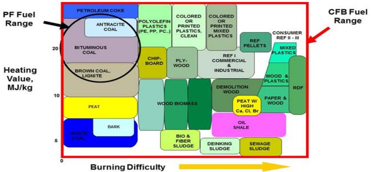
**Figure 4. Fuel Range Comparison for CFB vs PC**
